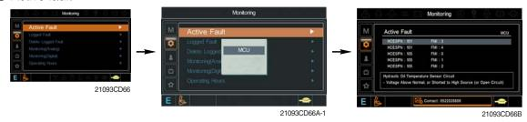
$\cdot\,$  The active faults of the MCU can be checked by this menu.
