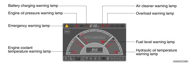
Each warning lamp on the top of the LCD pops up on the center of LCD and the buzzer sounds when the each warning is happened. The pop-up warning lamp moves to the original position and blinks when the select switch is pushed. And the buzzer stops.
